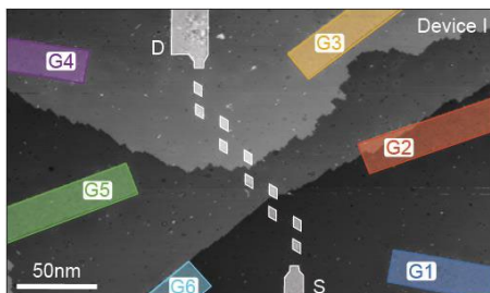
A scanning tunnelling microscope image of a 10-quantum dot quantum analogue simulator – mimicking a polyacetylene molecule
